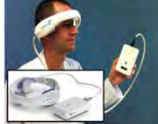
Figure 1. A. Operator-independent ultrasound device. B. The patient placed a head-mounted display (HMD) on his head. The HMD displays the ultrasound image of the brain. C. The patient placed a head-mounted display (HMD) on his head. The HMD displays the ultrasound image of the brain.
